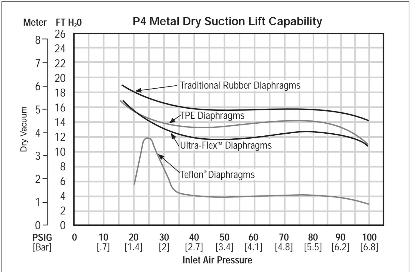
Suction lift curves are calibrated for pumps operating at 1,000' (305 m) above sea level. This chart is meant to be a guide only. There are many variables which can affect your pump's operating characteristics. The number of intake and discharge elbows,
