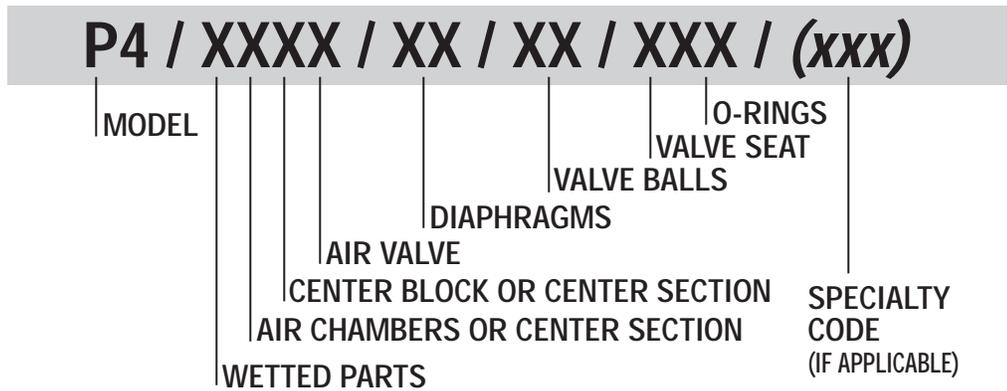
In the case where a center section is used instead of a center block and air chambers, the designation will be as follows: Acetal = LL
