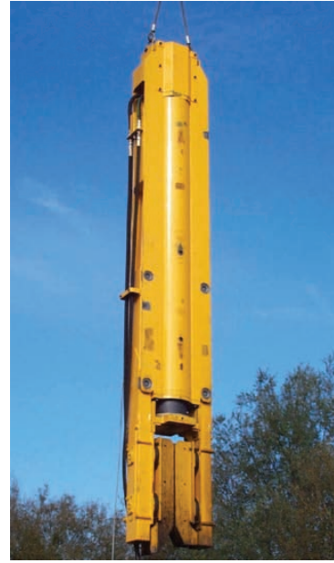
Above: Various SL30 Hammers fitted with legs and inserts for diving sheet piles. All are shown in crane suspended operation and powered by BSP Power Packs.
