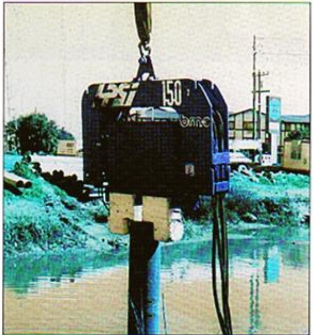
Model 150 w/50 ton caisson clamp assembly.
