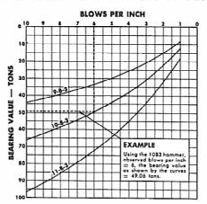
Pile static load bearing curves for McKiernan-Terry 9B3, 10B3 and 11B3 double-acting pile hammers. The curves are derived using the Engineering News Formula:
