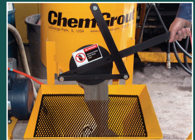
Mix tank's large slide gate allows for an easy transfer of material.
