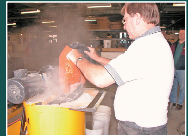
Twenty-two gallon mix tank allows for a batch size of up to 3-50 lb. bags.
