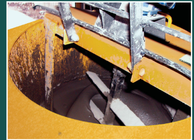
Three tough steel mixing blades thoroughly blend material providing a uniform mix.
