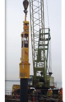
The CX range of piling hammers are designed to operate from standard USA leads or crane suspended. They are suitable for driving a wide variety of bearing and sheet piles. The hammers have the following important features.
