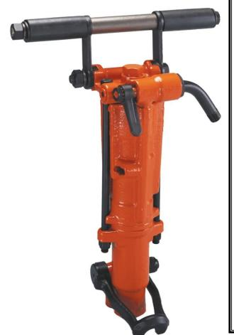
The APT Model 137 Rock Drill is a versatile midsize Rock Drill used in general construction, utility work, and plant maintenance. It is designed for drilling through granite, hard faced rock, quarry drilling and for drilling secondary holes for blasting. It can also be used in conjunction with dowel hole drilling machines. The Model 137 is adaptable to wet drilling application by attaching the APT valve, wet tube and swivel assembly.
