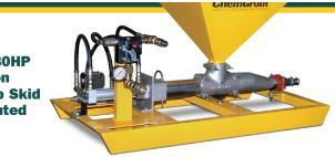
Complete grouting systems combine the CG-030 piston pump with a high efficiency paddle mixer to provide a continuous output of material. Both mixer and pump are equipped with their own variable speed control.
