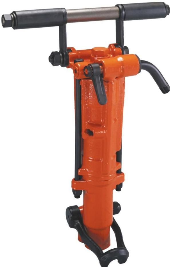
The APT Model 137 Rock Drill is a versatile midsize Rock Drill used in general construction, utility work, and plant maintenance. It is designed for drilling through granite, hard faced rock, quarry drilling and for drilling secondary holes for blasting. It can also be used in conjunction with dowel hole drilling machines. The Model 137 is adaptable to wet drilling application by attaching the APT valve, wet tube and swivel assembly.
