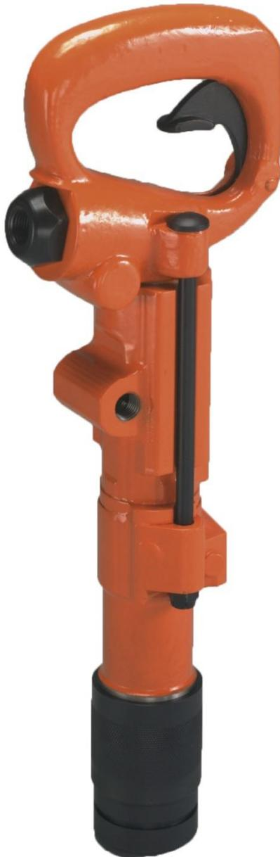
Weighing only 9 lbs, the APT Model 109 Rock Drill & Utility Drill is the lightest tool American Pneumatic makes. It is the ideal tool for drilling holes for anchor bolts as well as for small dowel hole drilling. The stop rotation feature easily converts the tool from a drilling machine to a percussion only tool.
